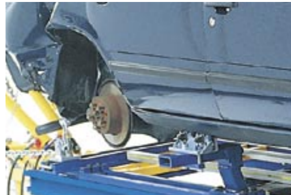
Performance Track 2500 uses existing Car-O-Liner holding accessories, specially clamps and truck repair system.
